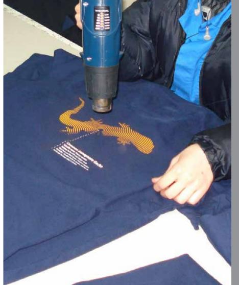
AZRAQ Silk Screen Printing Workshop Silk printing is the art of printing designs on a screen of silk, with blank areas coated with an impermeable substance, and ink is forced through the silk onto the printing surface.
